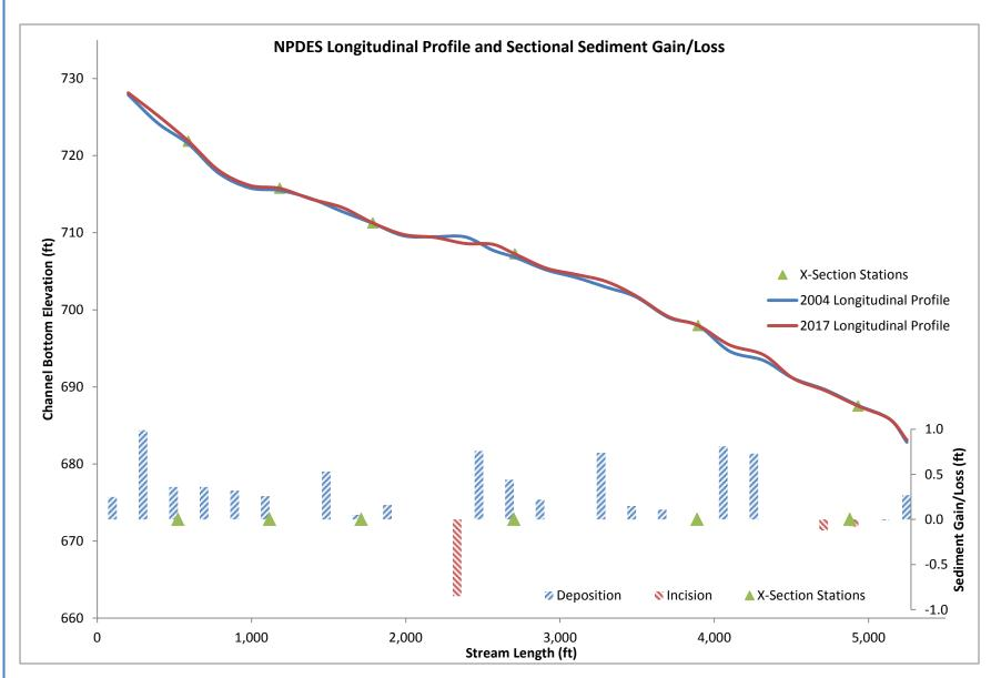
Figure 18: Comparison of Longitudinal Profile and Sectional Deposition/Incision from 2004 - 2017
