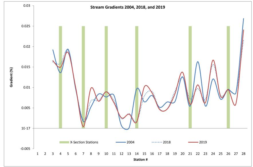
Figure 17: Stream Gradient Change from 2004 – 2019
