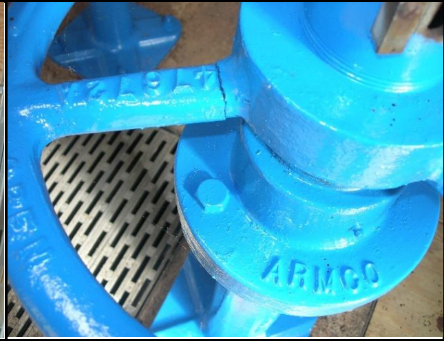
Image 50: Close-up on one of the multiple slide gate operator's broken spoke
