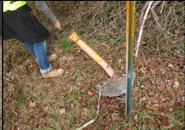
Image 54: Damage to observation well #11
