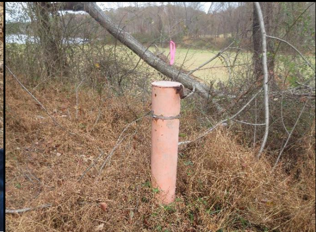
Image 52: Locked observation well, ASW outside slope
