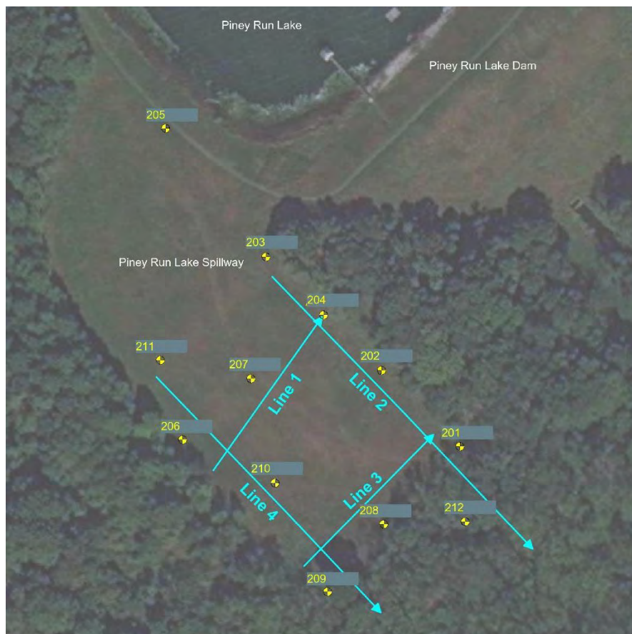
Figure 5: Seismic refraction survey lines
