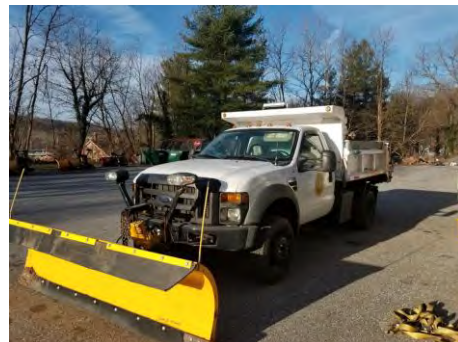
Ford Dump Truck with electronic salt spinner; 10-year anticipated replacement, or as-needed.
